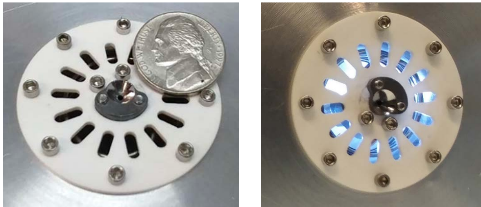
Figure 8: Fabricated micro-nozzle installed in the ceramic insulator plate and MVP housing: (left) shown with a coin for scale, and (right) shown with light shining through backside to illuminate the installed superheater assembly behind the nozzle.
