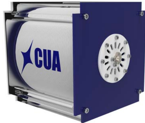
Figure 2. Solid model rendering of flight-like MVP assembly. Note that the outside housing is rendered as a clear plastic, whereas the actual unit will have an aluminum housing.
