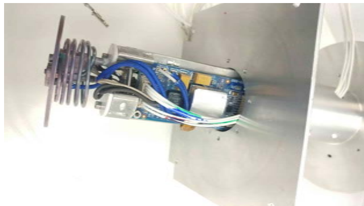
Figure 9. Final core assembly (left side of image) during insertion into and integration with fiber spool (right side of image).
