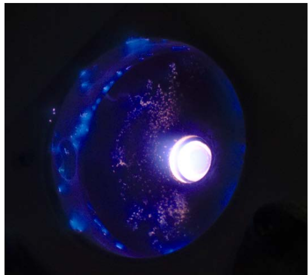
Figure 26. Thruster firing with electromagnets turned on with current flow in the “reverse” direction.
