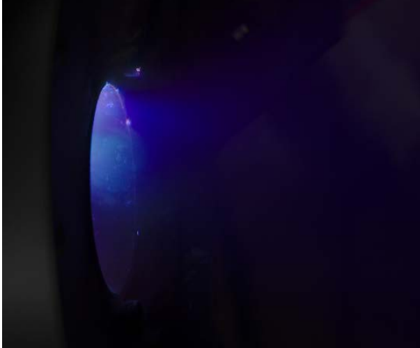
Figure 23. Thruster firing with electromagnets turned on with current flow in the “forward” direction. Camera is looking down from above.
